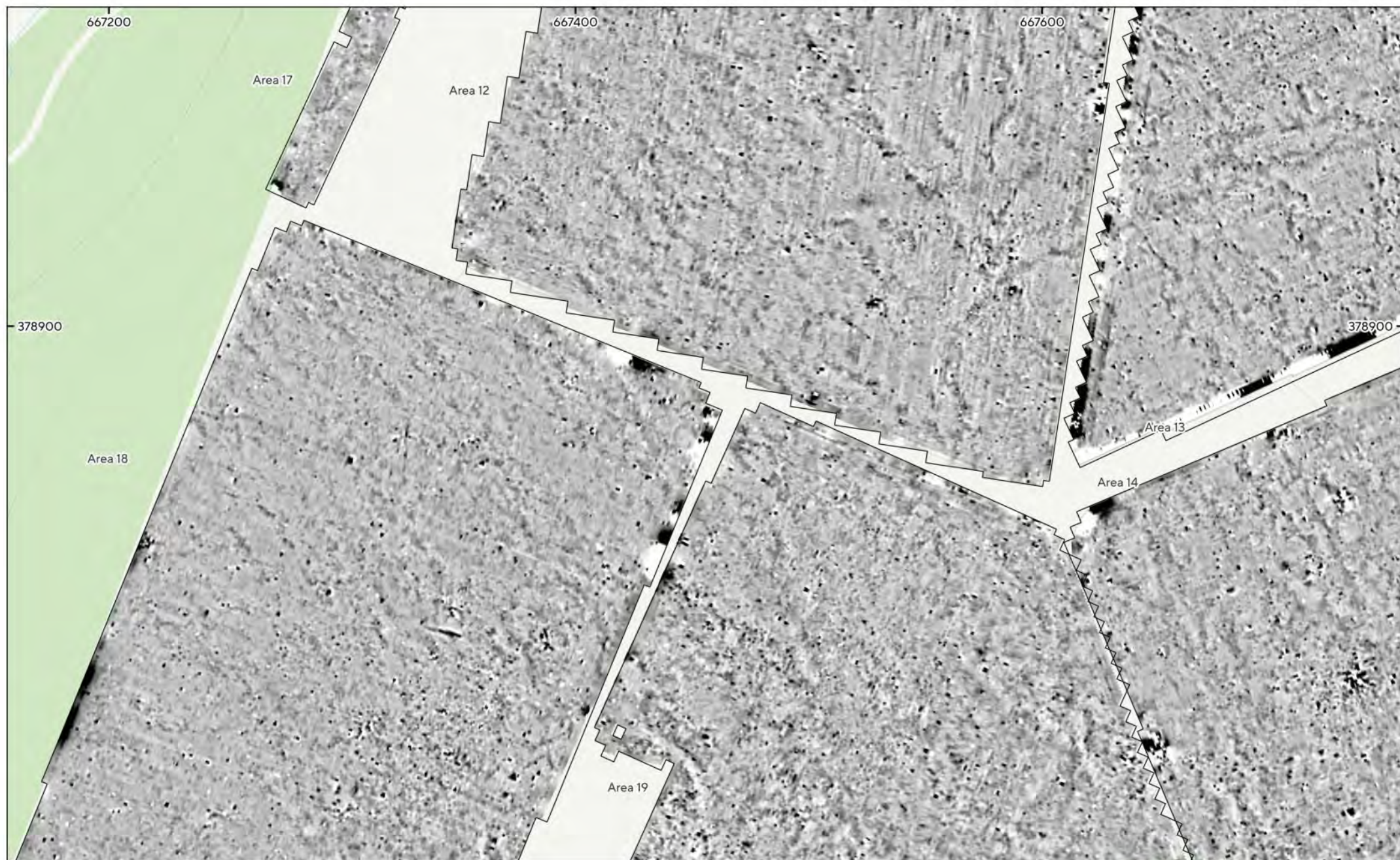
MSNT1874 - Bowshiel, Scottish Borders Figure 51 - Magnetic Gradient (Area 13 & 14 (South), 12 & 17 (East), 18 & 19 (West)) 1:1,500 @ A3 © Magnitude Surveys 2024 Contains Ordnance Survey data © Crown Copyright and database right 2024
